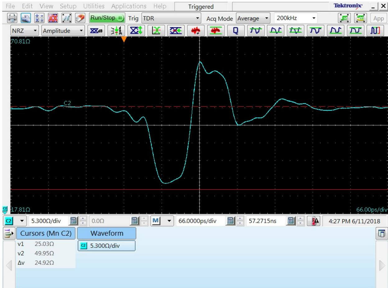
When considering that the limit of the TDR is 28ps in the best case, the fact that the dip doesn't quite reach 25ohms is easy to understand. The experimental results match very well the simulated one.
