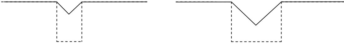
The stub on the left is a length  $L$  and the right is a stub  $2L$ . The depth of the stub response on the right will be deeper, since the same slope will travel longer along the voltage axis as its period is longer. This creates a linear relationship between stub length and TDR response dip, but still highly susceptible to changes in bandwidth and rising edge.
