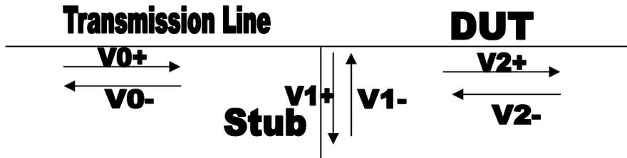
The system has 5 unknowns. The transmitting signal on the transmission line is the source which is a step function. The current can be assumed to be zero at the end of the stub and DUT since it's an open circuit. The voltages on the middle node must be equal. The following set of equations describes the system.
